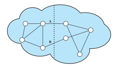
Figure 19.7 Packet-Switching Network Subject to Oscillations
