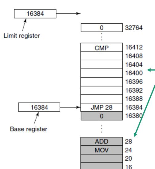
Two processes, each has its own logical address spaces starting at 0, which are mapped to separate physical address spaces starting at the addresses in their respective relocation (or base registers)
