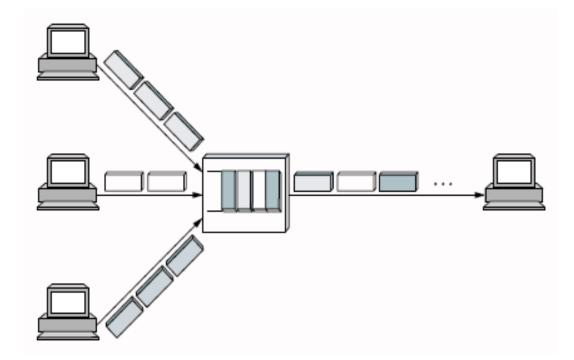
A switch multiplexing packets from multiple sources onto one shared link.
