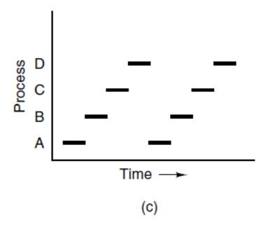
In a single processor core system, only one program is active at once (pseudoparallelsim) [Figure 2-1(c) in Tanenbaum & Bos, 2014]
